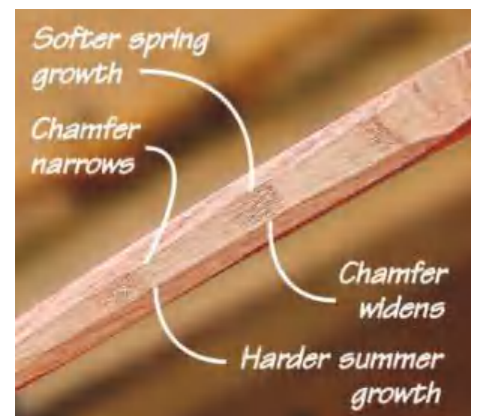
▲ Pic.4 Variations in the wood's hardness caused these irregularities
